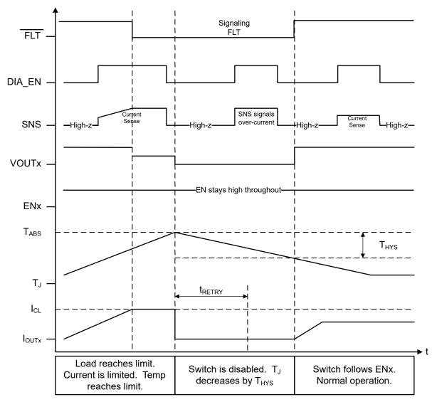
Figure 9-15. Current Limit – LATCH = 0
