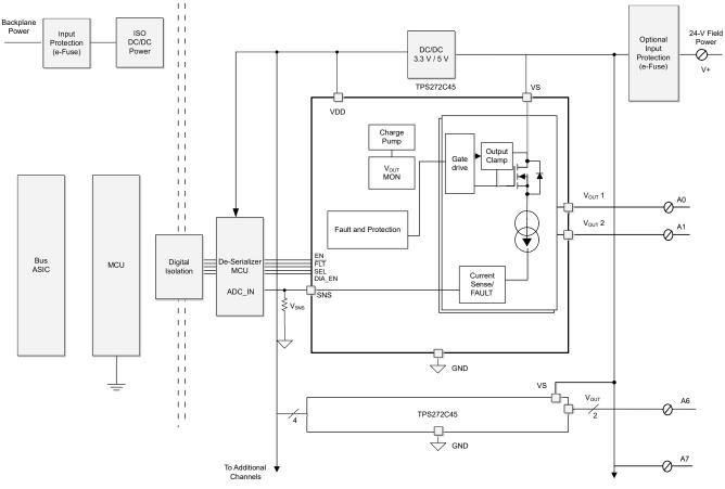
Figure 10-3. Block Diagram for PLC Digital Output Module
