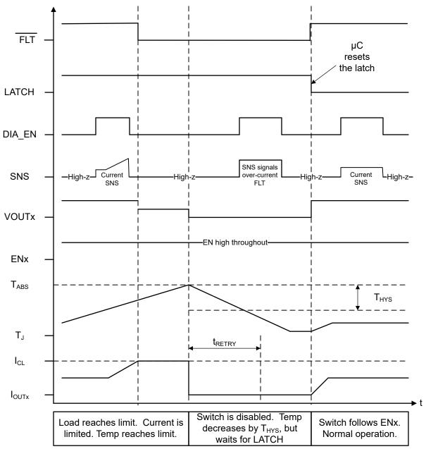
Figure 9-14. Current Limit – Latched Behavior
