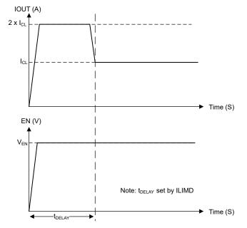
Figure 9-3. Inrush Current Control (Case 2) With a Shorted Load
