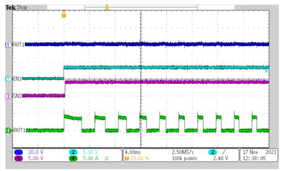
Figure 10-8. Permanent Short Behavior (R<sub>ILIM</sub> = 10 k, V<sub>S</sub> = 24 V, Delay = 6 mS)
