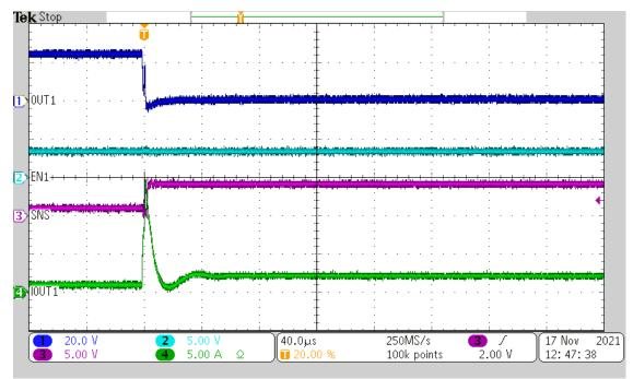
Figure 10-9. On-State Short Circuit (R<sub>ILIM</sub> = 10 k, V<sub>S</sub> = 24 V)
