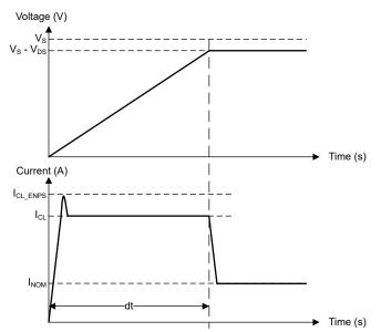
Figure 9-7. Enable into Short-Circuit Behavior
