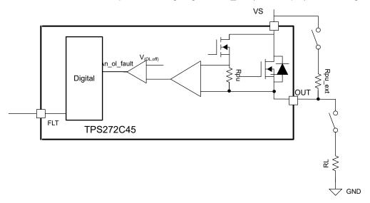
Figure 9-17. Open-Load Detection Circuit
