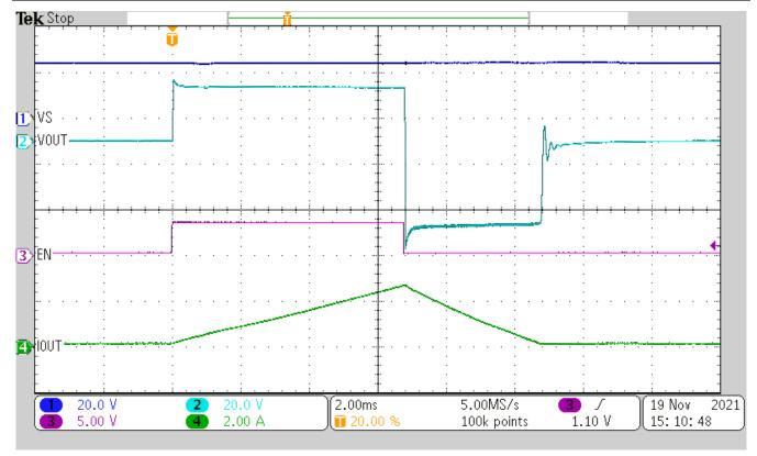
Figure 9-10. TPS272C45 Inductive Discharge (40 mH)
