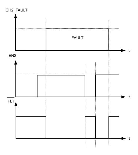
Figure 9-12. FLT Pin Behavior (Versions A, B, C)
