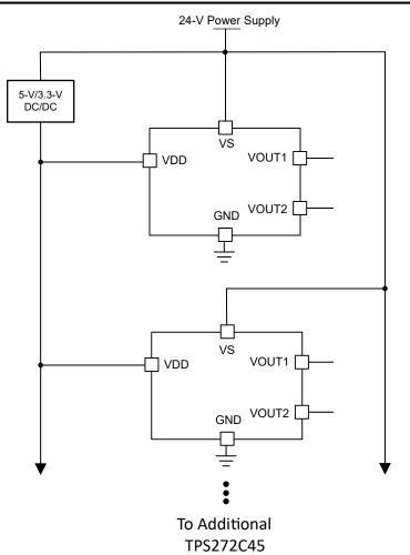
Figure 9-6. Secondary Low Voltage Supply Schematic
