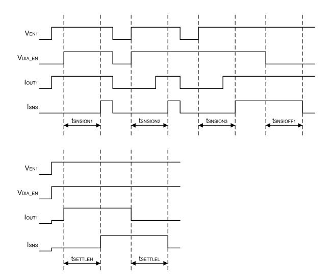
Rise and fall times of control signals are 100 ns. Control signals include: EN, DIA\_EN, SEL SEL pin must be set to the appropriate value.
