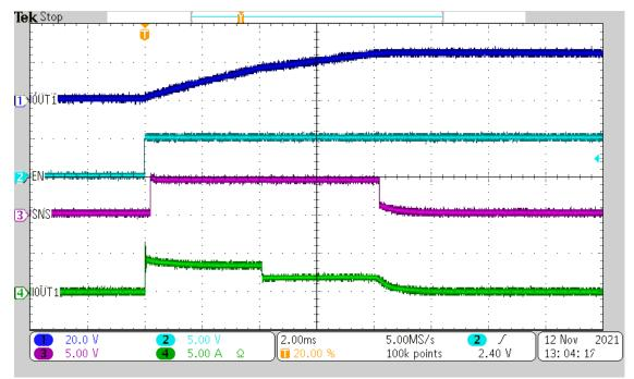
Figure 10-4. TPS272C45 Capacitor Charging
