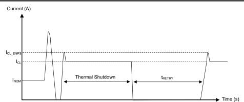
Figure 9-8. On-State Short-Circuit Behavior
