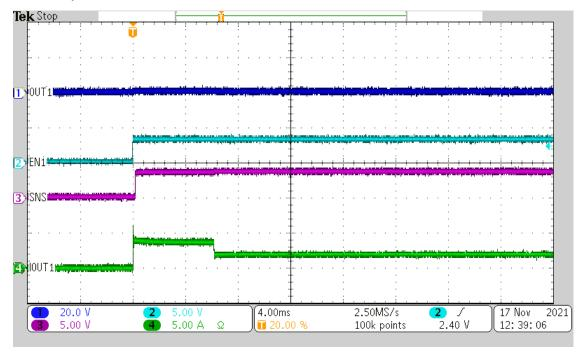
Figure 10-6. Enabling Into Short (R<sub>ILIM</sub> = 10 k, V<sub>S</sub> = 6 V, Delay = 6 mS)
