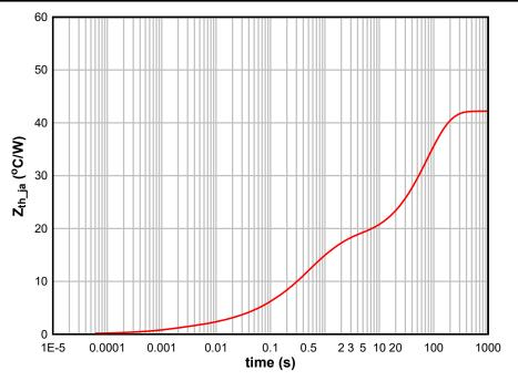
Figure 10-2. TPS272C45 Transient Thermal Impedance
