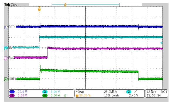
Figure 10-7. Enabling Into Short (R<sub>ILIM</sub> = 10 k, V<sub>S</sub> = 24 V, Delay = 6 mS)
